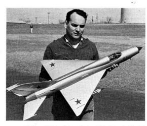
Model could have been designed for Dynajet, but it is noisy, requires heavy insulation, can't be throttled. You won't see the propeller in flight anyway!
